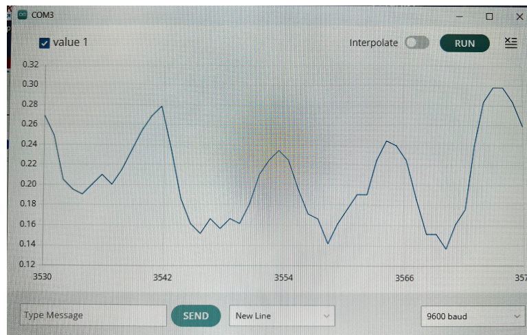
Figure 3: Observed arduino voltage output using the C++ arduino IDE code to measure the PIN 3 input. A conversion formula was implemented in the code to verify the volts/bit measurement ( 5/1023 ).
