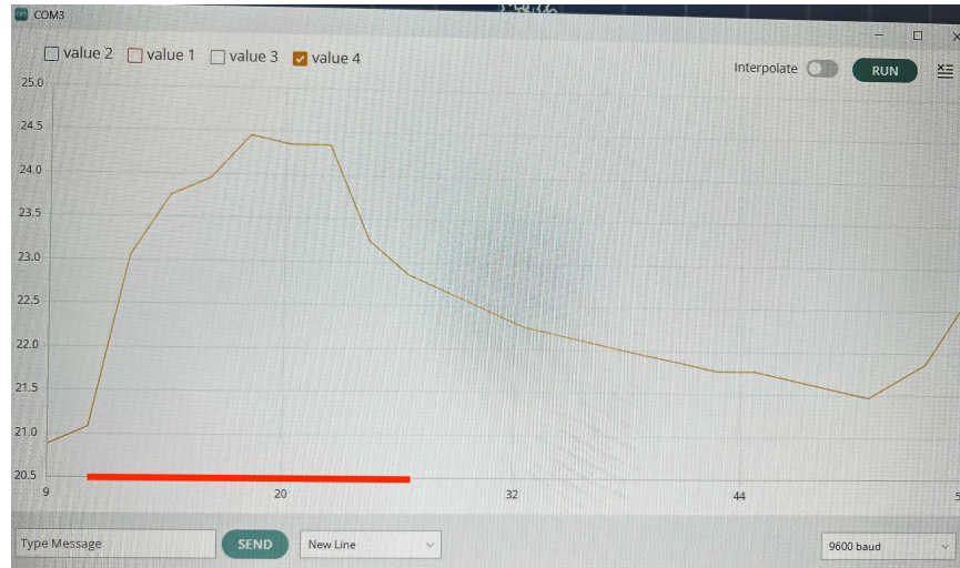
Figure 4: Arduino IDE screen capture of the temperature output reading when pinching the thermistor. The lower red line annotation indicates the approximate time of when the thermistor was pinched, decreasing the resistance in the circuit.
