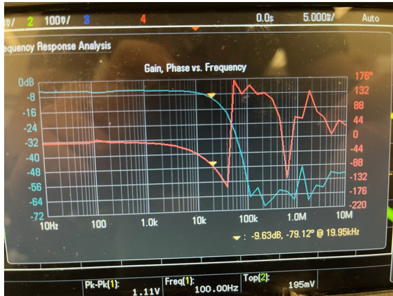
Figure 6: Bode plot of the frequency analysis given to the circuit via the oscilloscope. The -3db cutoff was located around 20\text{ kHz} . The screen capture instead of actual plot is a result of running out of time (we messed up the first plot).
