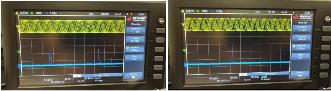
Figure 2: (Left and right) oscilloscope screen captures of analog pulses created by the LED voltage divider at 9.4 and 9.3 VPP wavegen inputs, respectively. Pulses are faint, but they exist.
