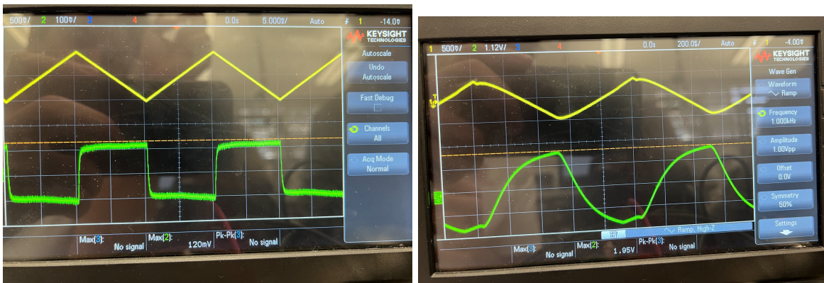
[Figure 2]: scope image captures when a 100nF capacitor is placed in parallel to the resistor. As frequency of the wavegen is increased, the smoothing of the attack/decay of the output is increased, which suggests that the capacitor reduces the rate of change of voltage slightly.
